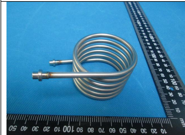
Picture 33, Boiler water pipe
