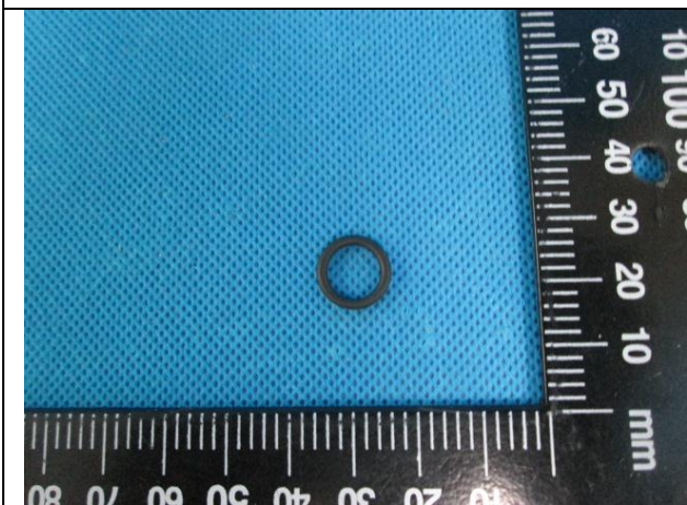
Picture 29, Gasket ring in self-priming valve/O-ring
